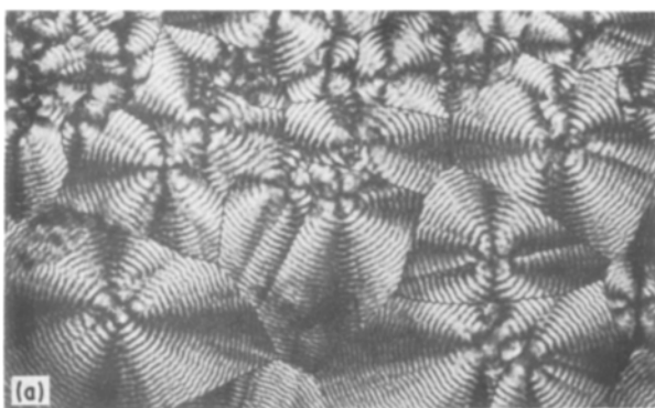
Figure 8 Optical micrographs of polymers (a) PE-1, (b) PE-3 and (c) PE-5 between crossed polarizers.
